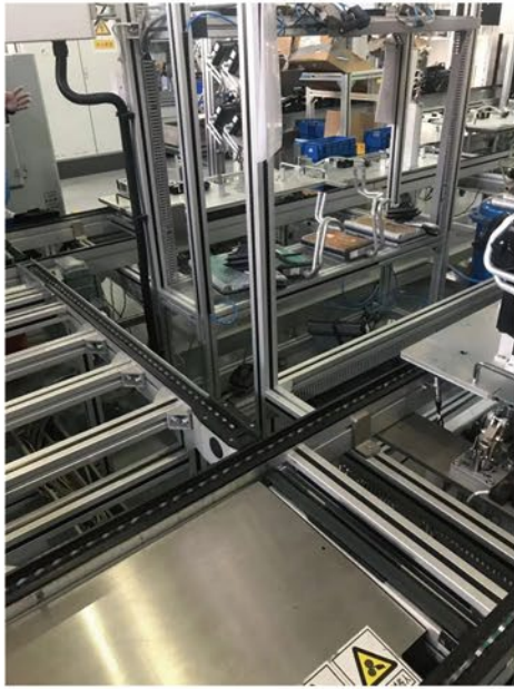
XI-TS2托盘输送机 XI-TS2 pallet conveyor
