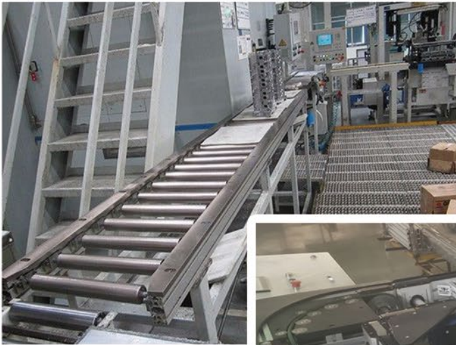
XI-RC/F无动力辊筒输送机 XI-RC/F non-powered roller conveyor
