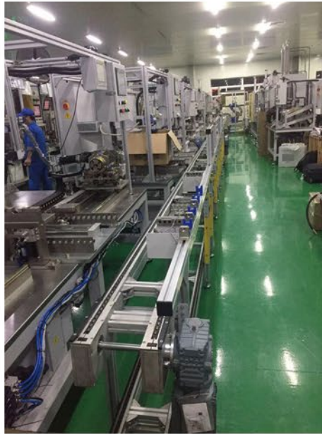
XI-TS4托盘输送机 XI-TS4 pallet conveyor
