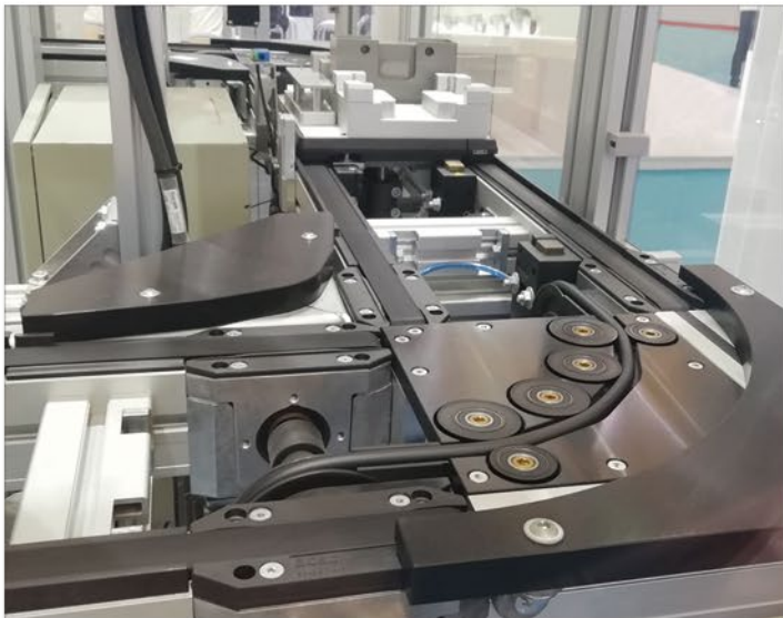
XI-CU90 90°圆带弯道机构 XI-CU90 90°round belt curve
