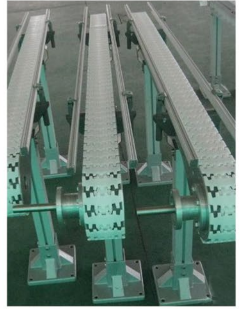
XI-TC顶板链输送机 XI-TC top chain conveyor
