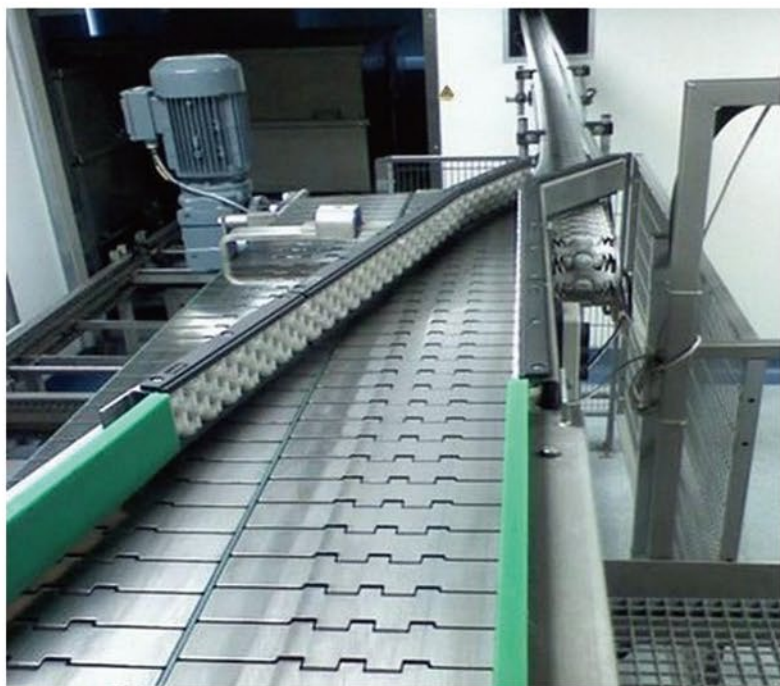
XI-TC顶板链输送机 XI-TC top chain conveyor
